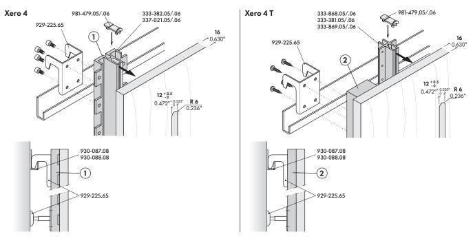
• Please note that the fixing set 929-225.65 cannot be attached to Xero 4T profiles. Panels with these profiles are to be attached to the wall e.g. with wedge gibs.
