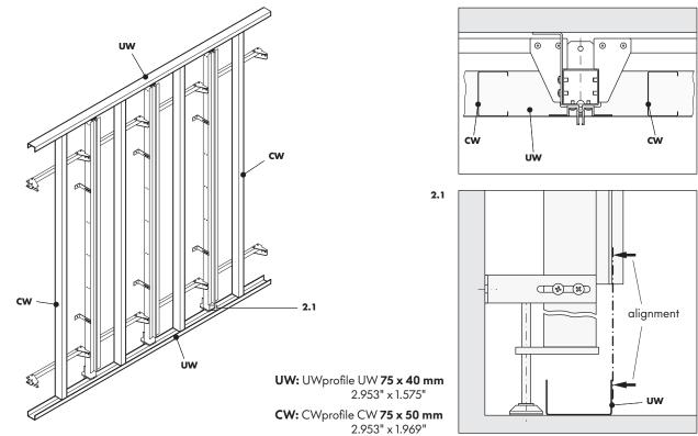
2.1 Set-up metal frame (UW- and CW-profiles): check that profiles are aligned with UW profile. The structure of the wall unit is designed for metal frames with a profile width of **75 mm**/2.953"
