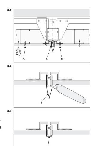
Screw the gypsum panels to the metal frame profile using dry wall screws A (e.g. Ø 3.9 x 19 mm/0.154"x 0.748").
